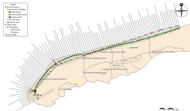
Figure 9. Map overview of the calculated retreat points. The map is coupled to a time navigator, which allows scrolling through time. The MorphAn overview also includes a layer that shows the normative retreat points.
