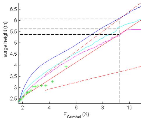
Figure 1: Gumbel plot of  $1 \cdot 10^{-4}$  year<sup>-1</sup> surges (at vertical dashed line). Surge levels based on model output are denoted in blue. Results of improved datasets are shown in cyan and magenta. Results based on extrapolation of measurements (green pluses). The solid red line shows the currently adopted probability of exceedance curve, the 95% probability interval is shown by red dashed lines.
