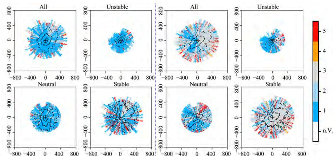
**Figure 7** Spatial distribution of the data quality for the latent heat flux at the NPCE-BJ site under different atmospheric stratifications during the monsoon season (left) and post-monsoon (right). Black isolines indicate the flux contribution for the sink area, with 50%, 80%, and 95% from inside to outside, respectively. '+' is the location of the BJ station
