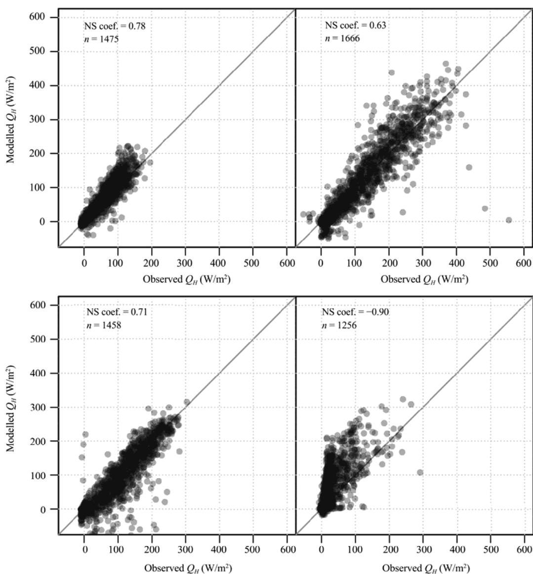
**Figure 9** Energy balance corrected fluxes vs. optimized model runs, subjected to gap-filling for the NPCE-BJ station; the sensible heat flux and the latent heat flux from left to right during the monsoon season (upper) and post-monsoon (lower);  $n$  is the number of available observations and  $NS$  is the Nash-Sutcliffe coefficient
