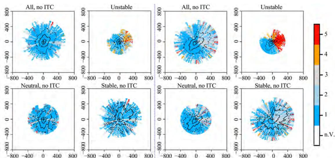
**Figure 6** Spatial distribution of the data quality for the sensible heat flux at the NPCE-BJ site under different atmospheric stratifications during the monsoon season (left) and post-monsoon (right). Black isolines indicate the flux contribution for the sink area with 50%, 80%, and 95% from inside to outside, respectively. '+' is the location of the BJ station
