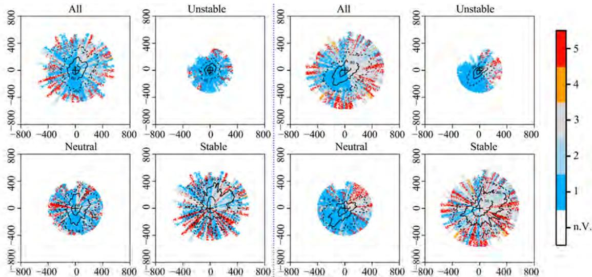
**Figure 8** Spatial distribution of the data quality for the carbon dioxide (CO<sub>2</sub>) flux at the NPCE-BJ site under different atmospheric stratifications during monsoon season (left) and post-monsoon (right). Black isolines indicate the flux contribution for the sink, with 50%, 80%, and 95% from inside to outside, respectively. '+' is the location of BJ station
