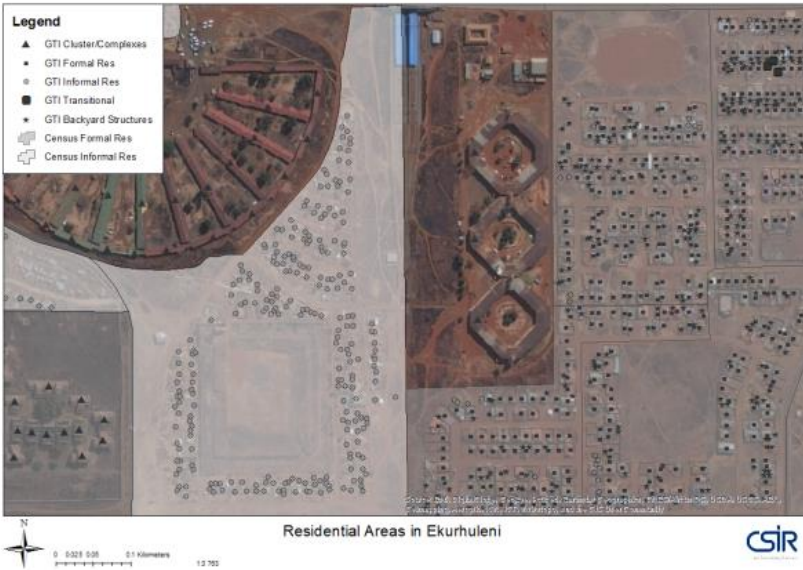
Figure 6: An overlay of small area boundaries on GTI building-based land-use point data for validation of Census 2011 dwelling type data
