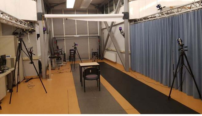
Fig. 4. Vicon system with eight cameras. A table in the middle of cameras was used as a support during the static experiment. All the data were preprocessed with the Vicon Nexus 2.10.2 software.
