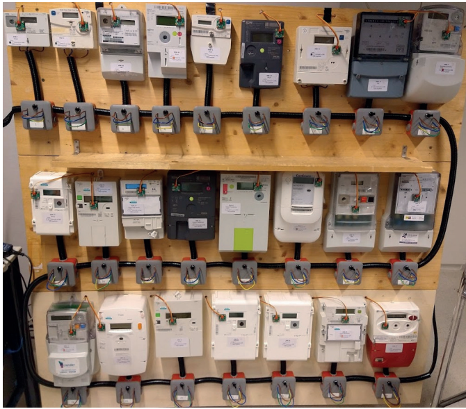
Fig. 4. Picture of the 24 static energy meters used in the setup
