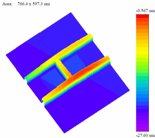
Figure 6: A 3-Dimensional surface profile of doubly clamped H-shaped piezoelectric AlN thin film suspension device using an ATOS white light interferometer.
