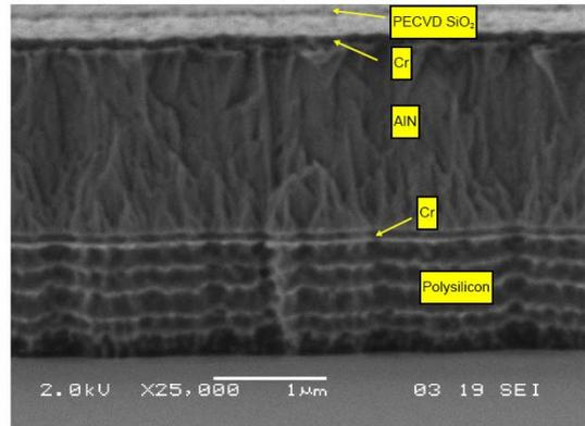
Figure 4: Anisotropically etched (002) textured AlN thin film between Cr layers after Bosch process.
