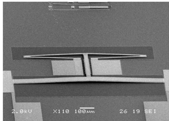
Figure 5: A doubly clamped unimorph piezoelectric microstructure with a spring element.
