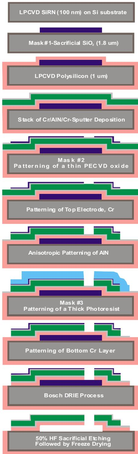
Figure 3: Fabrication process flow of the AlN thin film piezoelectric microstructures.
