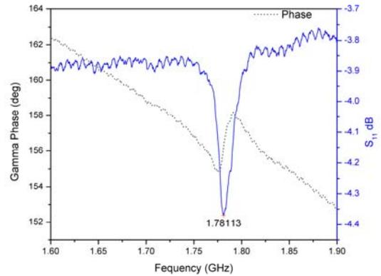
Figure 7: Measured reflection coefficient,  $S_{11}$  (-4.4 dB) on the clamped resonating beam of dimension (990 x 30)  $\mu\text{m}^2$  showing a resonant frequency of 1.74GHz.
