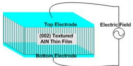
Figure 1: A simple AlN unimorph piezoelectric thin film resonating structure.
