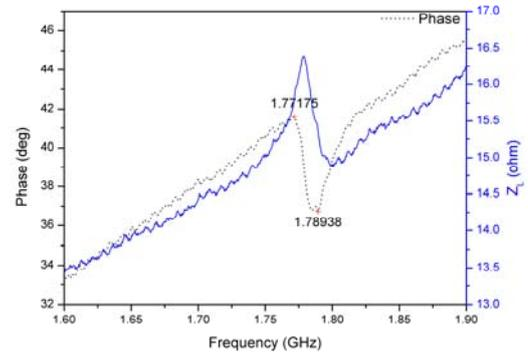
Figure 8: Narrow band impedance and phase response with resonant and anti resonant frequencies at 1.771 and 1.789 GHz respectively with a bandwidth of 13.5MHz.
