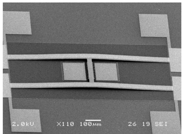
Figure 6: Doubly clamped H-shaped piezoelectric AlN thin film suspension device with patterned top and bottom Cr electrodes for electrical probing.
