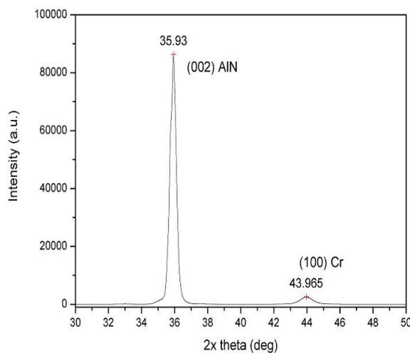
Figure 2.: XRD spectrum showing clear (002) diffraction AlN and a minor intensity peak of Cr.
