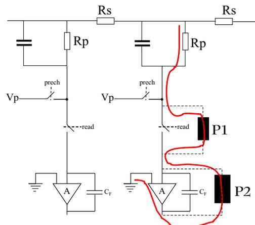
Fig. 9. Current path in the capacitive fingerprint sensor.
