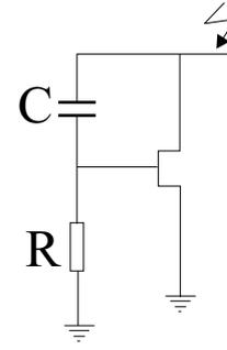
Fig. 10. Gate coupled TFT.
