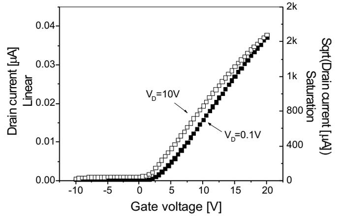
Fig. 5. Transfer characteristics  $I_D/V_G$  under different drain voltages  $V_D=0.1, 10$  V of a TFT with  $W/L=100/12$ .
