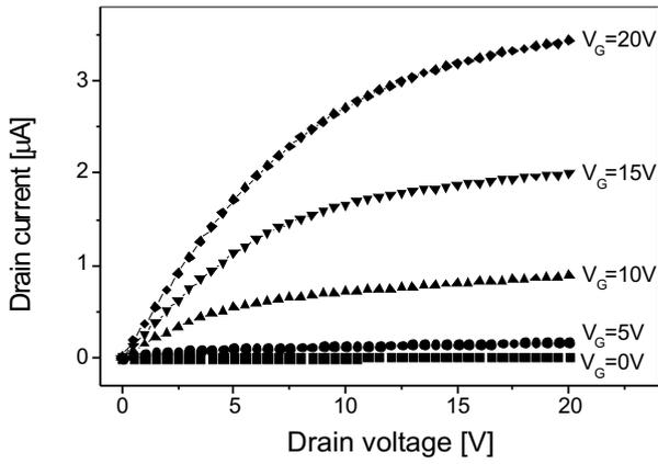
Fig. 4. Output characteristics  $I_D/V_D$  under different gate voltages  $V_G=0, 5, 10, 15, 20$  V of a TFT with  $W/L=100/12$ .
