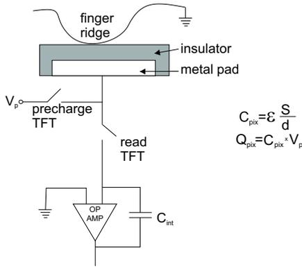
Fig. 2. Schema of the capacitive fingerprint sensor.
