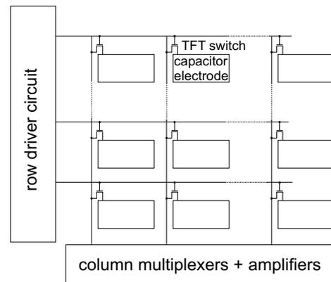
Fig. 1. A simplified schematic diagram of the sense elements together with associated addressing circuitry.
