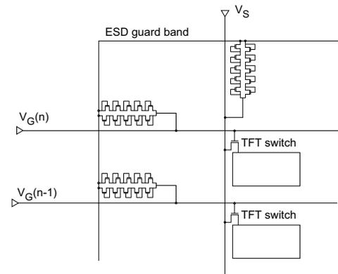
Fig. 7. TFT's chains in the fingerprint sensor.
