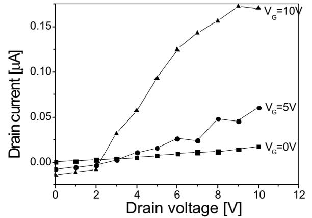
Fig. 6. Output characteristics of a TFT switch in the fingerprint sensor matrix.
