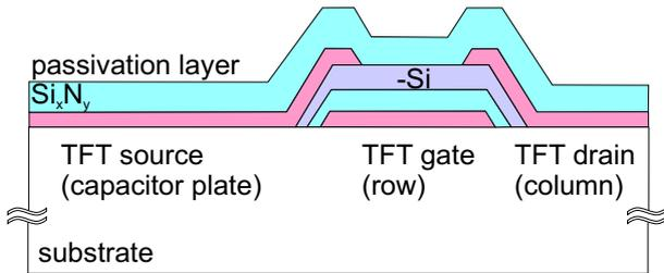
Fig. 3. Cross section of a pixel in the capacitive fingerprint sensor.
