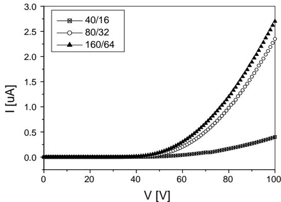
Fig. 8. Measured characteristics of TFT's chains with different channel widths and lengths.
