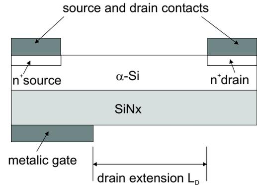
Fig. 11. High voltage TFT.
