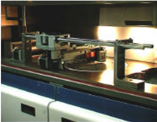
Figure 1. Ink-jet printing mechanism fits inside the Sinterstation 2000 machine
