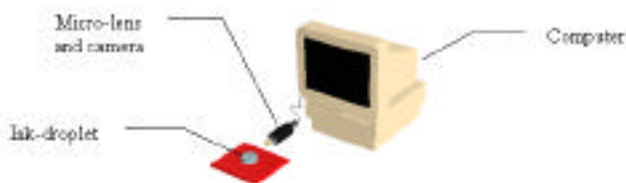
Figure 3. Apparatus used for a direct measurement of contact angle
