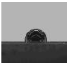
Figure 4. A magenta ink drop on the surface of Duraform powder
