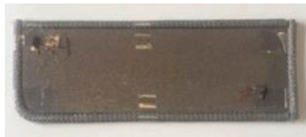
Fig. 4. Extra gasket placed around the harder nature materials for better contact between the MUT and the aperture
