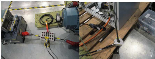
Figure 3. Photo of the set-up for common mode current measurement (a) input to converter, (b) output to the motor
