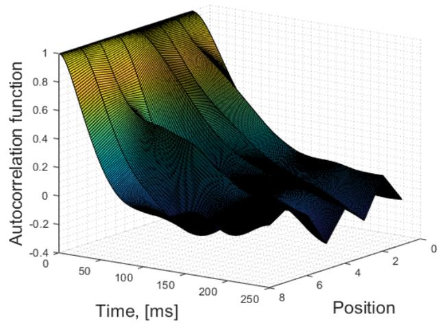
Fig. 6 Autocorrelation function calculated for eight different measurement positions at 700 MHz in 250 ms.
