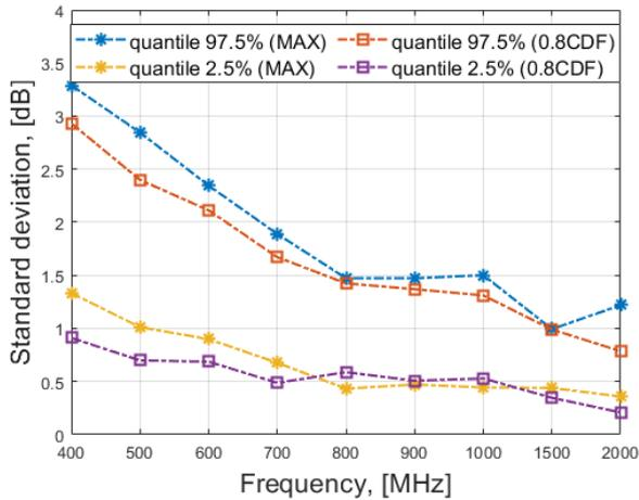
Fig. 9. Typical standard deviation of maximum (MAX) and quantile-80% (0.8CDF) levels into the UT-VIRC. Results refer to a population of 45 independent test and fixed observation time of 2 s.
