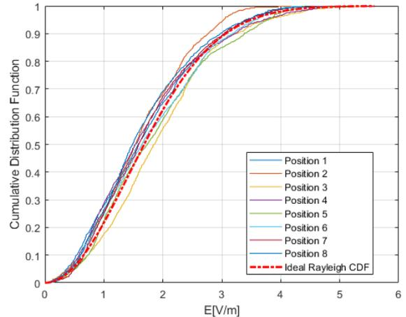
Fig. 3. CDFs of the measured field samples (dataset size is 2000 samples) show agreement at 2000 MHz with the ideal Rayleigh CDF.
