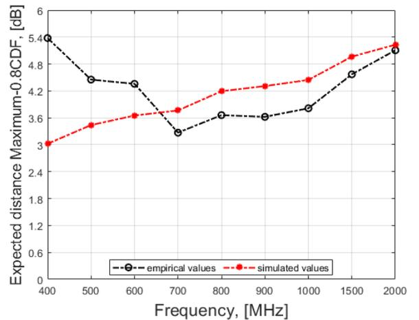
Fig. 10. Simulated (red curve) vs. measured (black curve) values of the distance between the quantile-80% (0.8CDF) and the maximum levels. Measurements refer to averaged data over 45 different test with eight dataset of 2000 samples. The number of uncorrelated samples used for the simulated dataset refers to Fig. 7.
