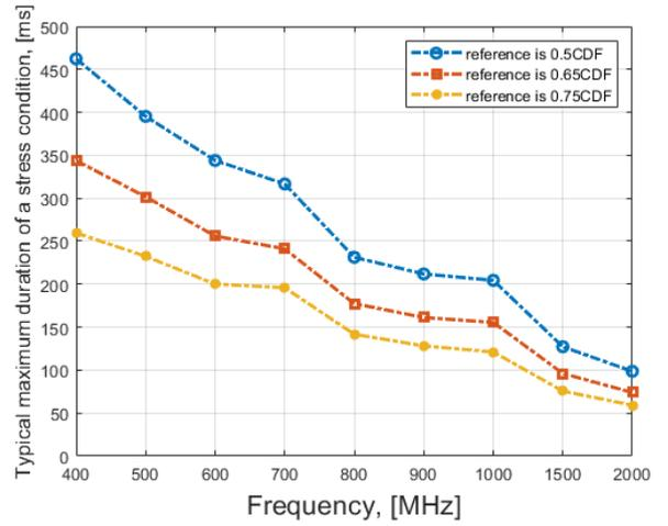
Fig. 12 Typical temporal length of the electromagnetic field strength level above the quantiles-50%,-65% and -75%. The dataset size is 2 s.
