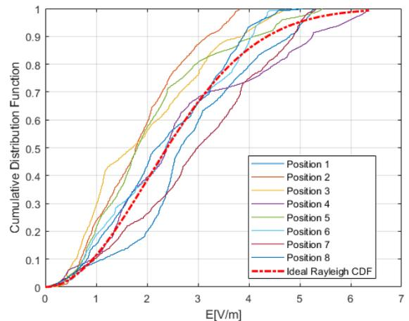
Fig. 4. CDFs of the field samples measured at 600 MHz and for each measuring position. The dataset size is 2000 samples.
