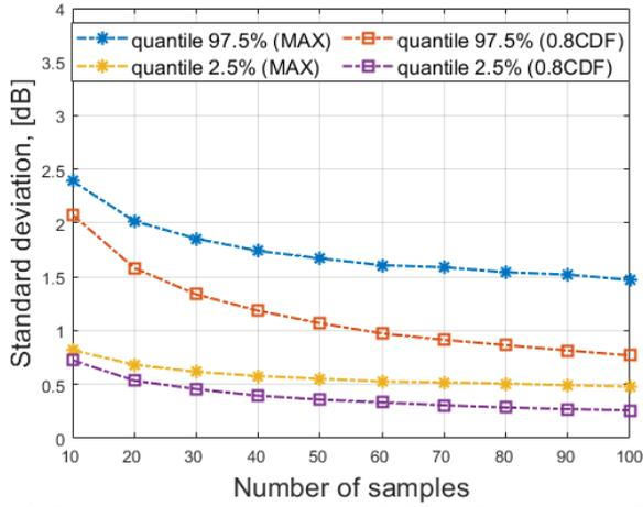
Fig. 8. Typical standard deviation range (95% confidence interval) for the maximum (MAX) and quantile-80% (0.8CDF) values among 10000 iterations of the MC program. The standard deviation is calculated for eight dataset with size (number of samples) of 10 to 100 samples.
