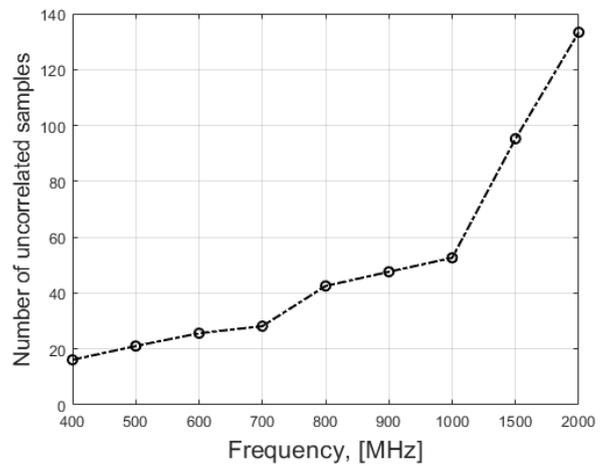
Fig. 7 Expected number of uncorrelated samples in datasets of 2 s vs. the working frequency.
