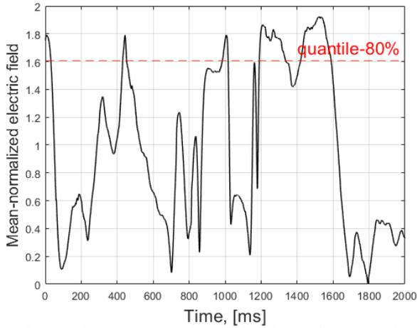
Fig. 1. Rectangular component of the electric field samples measured by a fast field probe in a VIRC. The sample values have been normalized with the dataset mean value.
