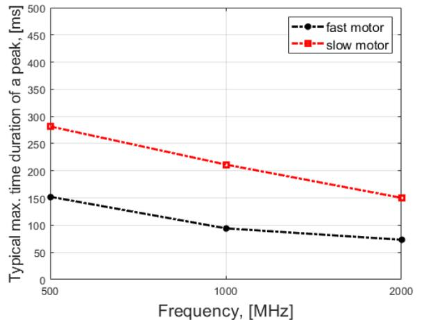
Fig. 13 Typical temporal length of the electromagnetic field strength level above the quantile-80%. Measurement taken for three working frequencies and in two configurations: VIRC shaken by one motor with fast (black curve) and slow (red curve) rotational speed.
