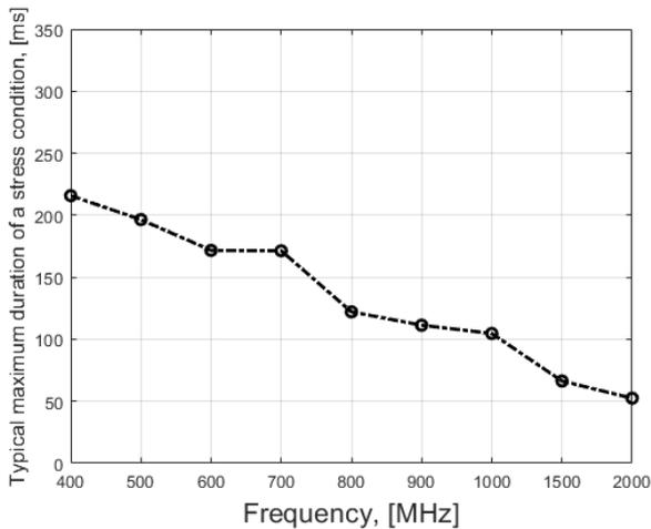
Fig. 11. Typical temporal length of the electromagnetic field strength level above the quantile-80%. The dataset size is 2 s.
