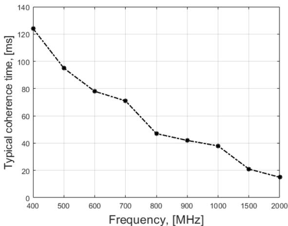
Fig. 5. Averaged value of the coherence time (among the eight measurement positions) vs. the working frequency.
