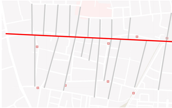
Figure 2: Example of neighborhood represented as a fishbone structure. The red line represents the main road and the grey lines the side-streets.
