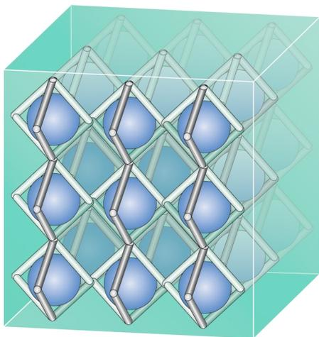
**Fig. 1 | A schematic of FLUID3EAMS.** A 3D solid scaffold (in light grey), produced using stereolithography or 3D printing, is filled with two immiscible fluids, which spontaneously self-organize as discrete particles (in blue) in a continuous phase (in green) to yield a 3D tri-material periodic structure. Figure adapted with permission from ref. <sup>1</sup>, Springer Nature Ltd.
