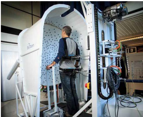
Figure 1: The Balance Test Room (BalRoom) set up consisting of support surfaces and a visual scene to apply sensory perturbations and rods on hip and shoulder level to apply mechanical perturbations to the human body.
