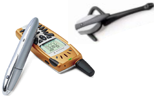
Figure 1 Bluetooth enables Chatpen and Headset to connect to mobile phone.
