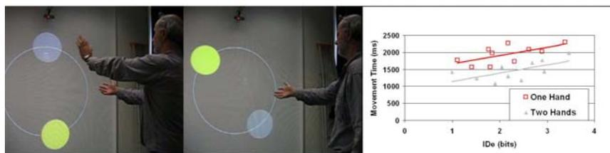
**Fig. 2.** Left: pointing a Fitts' law based ISO 9241-9 [3] target with a hand and selecting with another (*TwoHands*). Middle: pointing and selecting with *OneHand*. Movement time versus effective index of difficulty for *TwoHands* and *OneHand* devices.
