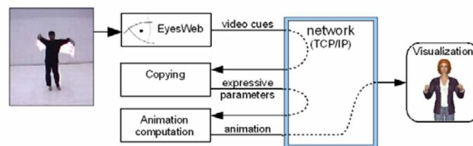
**Fig.1.** Overview of the system architecture modules. (1) *EyesWeb*: this module performs the automatic extraction of motion cues (e.g., amplitude, fluidity, velocity and acceleration of movement). (2) *Copying*: motion cues are mapped into agent's expressivity parameters. (3) *Animation computation* and *Visualization*: these modules, given the animation data in input, create a graphical representation of a virtual human.
