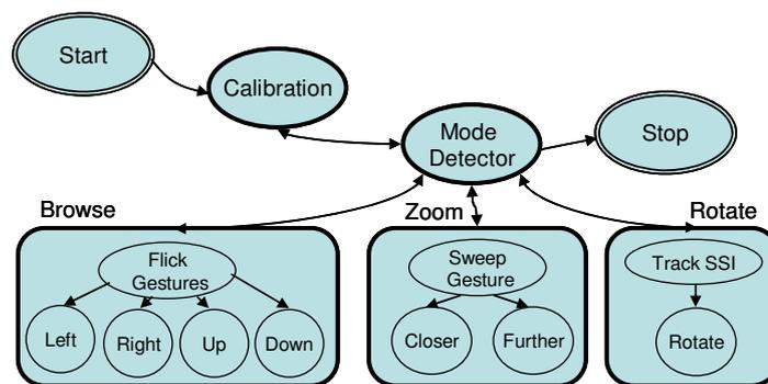
Fig. 2. State machine for the gesture-based medical browser
