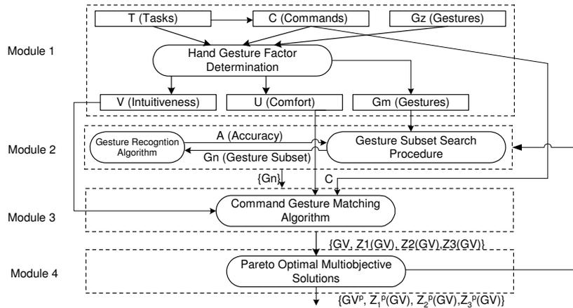
Fig. 1. Architecture of optimal hand gesture vocabulary
