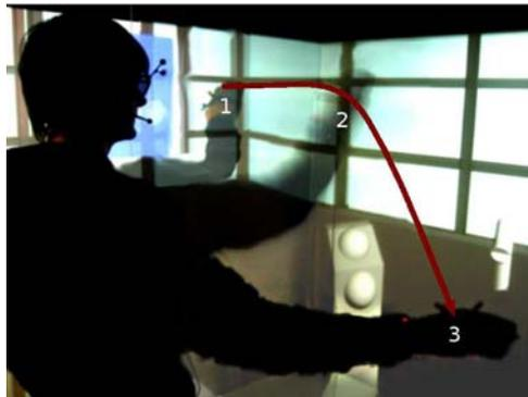
**Fig. 1.** Defining an object's shape via an iconic gesture, in this case a curved cylinder
