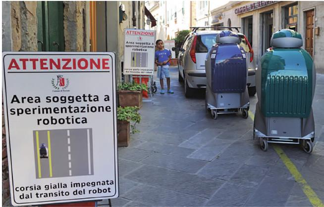
**Fig. 1.** DustCart from the DustBot project and its testing zone
