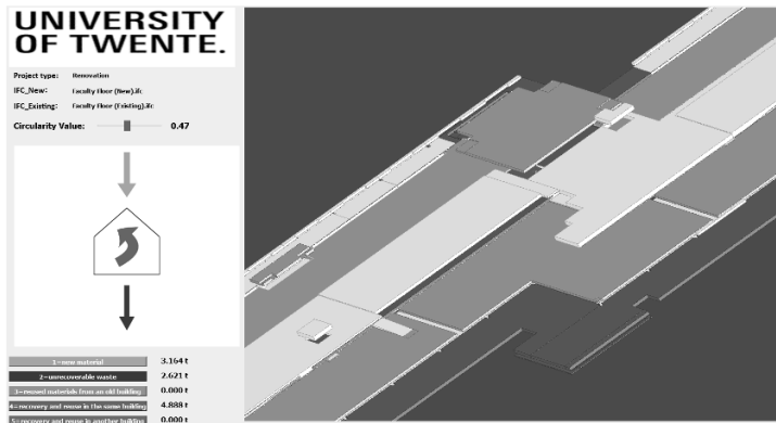
Figure 4: Assessment results of the renovation project (floor components) in the BIM-based tool (red represents waste; green shows reused entities in the same building; pink represents entities that compose of new materials)
