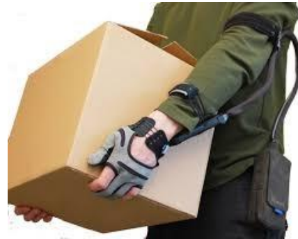
Figure 1. The Carbonhand System with soft-robotic glove, control unit worn on the hip and the cable connecting control unit and glove.
