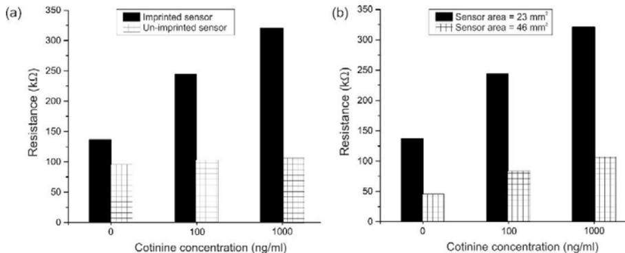
Figure 3: (a) Control experiment for an un-imprinted polymer film with IDE of 23 mm<sup>2</sup> (IDE1) surface area. The dc resistance of the un-imprinted polymer is measured for various concentration of cotinine (b) Sensor response of the cotinine imprinted MIP-CNT polymer film for various concentration of cotinine with IDEs of 23 mm<sup>2</sup> and 46 mm<sup>2</sup> surface area.
