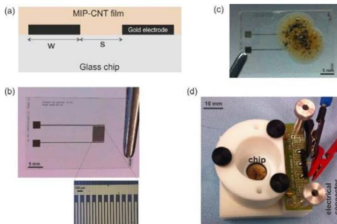
Figure 1: (a) Schematic of the cross-section of the IDE chip,  $w$  = width of planar electrode and  $s$  = spacing between electrodes (b) The top view of the gold IDEs on a glass chip and the magnified view of its fingers (c) The top view of the cotinine MIP-CNT polymer film deposited on the IDE chip (d) Snapshot of the sensor chip placed in a Teflon chemical cell with electrical connections.
