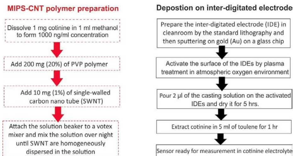
Figure 2: Scheme of the preparation of cotinine selective MIP and its deposition on the gold inter-digitated electrode array.
