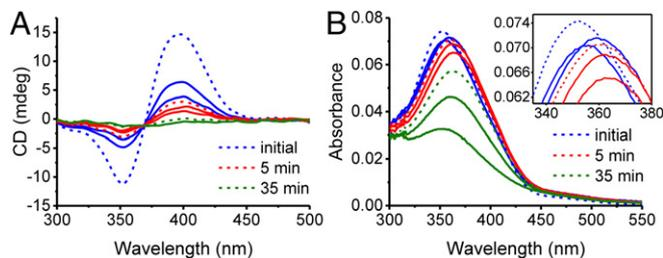
**Fig. 5.** Conversion of light into molecular and supramolecular strain. (A) Evolution of the CD spectra of tubules formed by **1** (2.5  $\mu\text{M}$  solution of **1** in water) as a function of the time upon irradiation (measured at 0, 1, 2, 5, 10, 20, 35, 50, and 60 min) with UV light ( $\lambda = 365$  nm). The disappearance of the CD signal after 35 min indicates that the tubules have disappeared. (B) Absorption spectral changes induced by irradiation with UV light.
