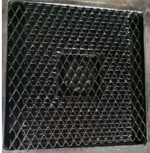
Figure 5.1 Flow geometry of the electrode compartment: Pt/Ti mesh on top, perpendicular flow field below, a manifold both for the inlet and for the outlet, all contained in plastic housing. The dark colour of the electrode originates from its use with the carbon-based slurry electrode.
