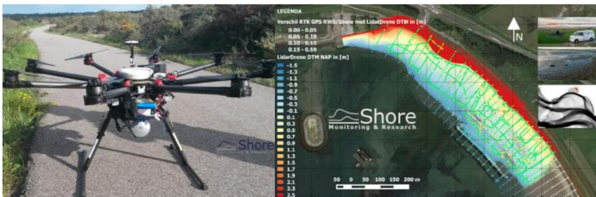
Figure 1. Left: the LiDAR drone. Right: LiDAR drone DTM in [m] RD NAP. Colours represent height and correspond to the colour bar in the legend. Height difference LiDAR-GPS indicated on DTM.
