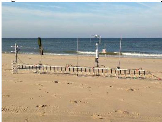
Figure 33: Saltation Detection System (SalDecS) installed at the beach south of Egmond aan Zee. The horizontal oriented array contains 32 sensors to measure small-scale spatiotemporal variability in saltation with a spatial resolution of 0.10 m and a frequency of 10 Hz.
