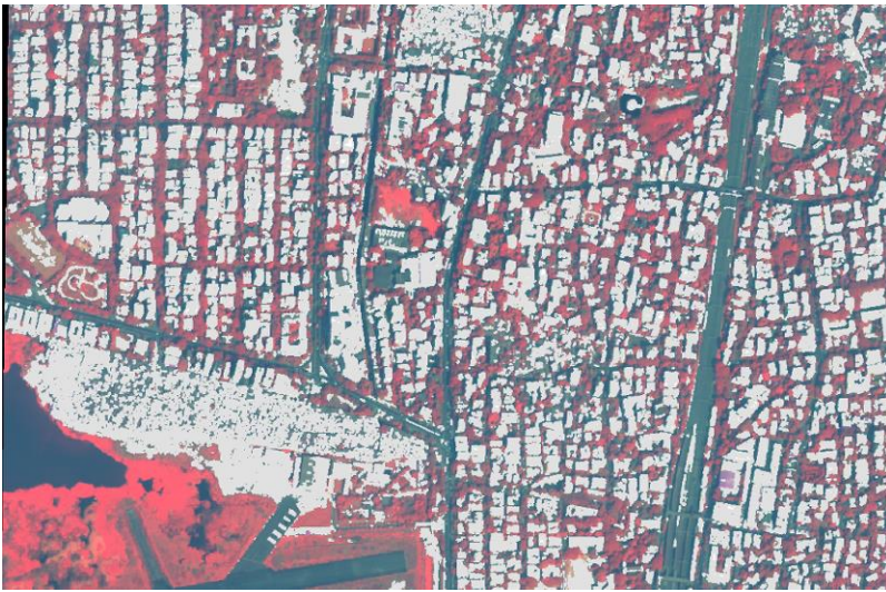
[fig. 6] Example of extracted building footprints: grey areas represent buildings footprint, on the back the image mosaic (FCC)
