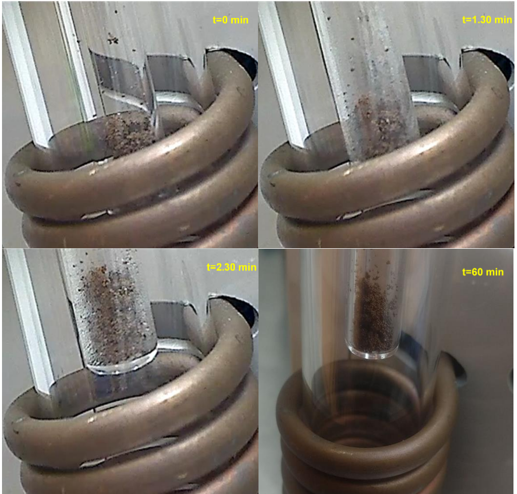
Figure S-4. The pictures from the AMF heating step to desorb water.
