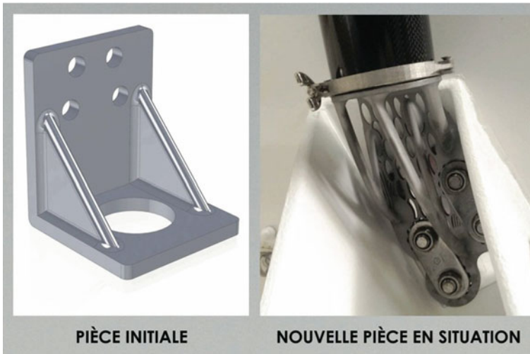
Fig. 6 On the left: initial part; on the right: optimized part ( source Volume—Fabrication Additive Dunod 2015)
