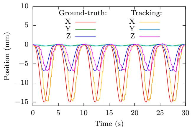
Fig. 5: Result of a representative experiment for the target tracking algorithm performance (case I). The motion described by (19) is applied to the gelatin phantom with a period  $T = 5$ s. Mean tracking error is 3.6mm for this experiment and reduces to 0.6mm after compensating for the delay of about 450ms introduced by data acquisition.
