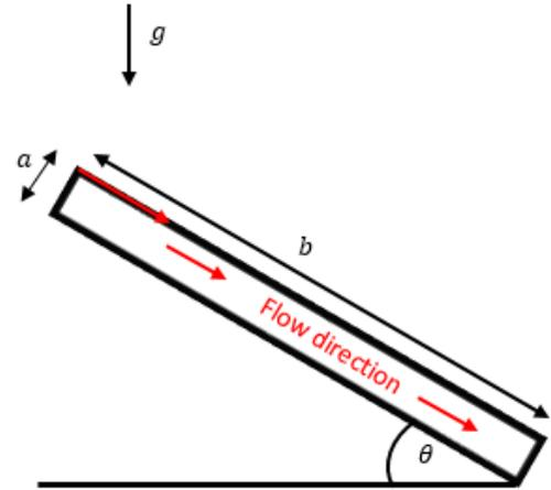
Fig. 1. Schematic of 2D rectangular microchannel
