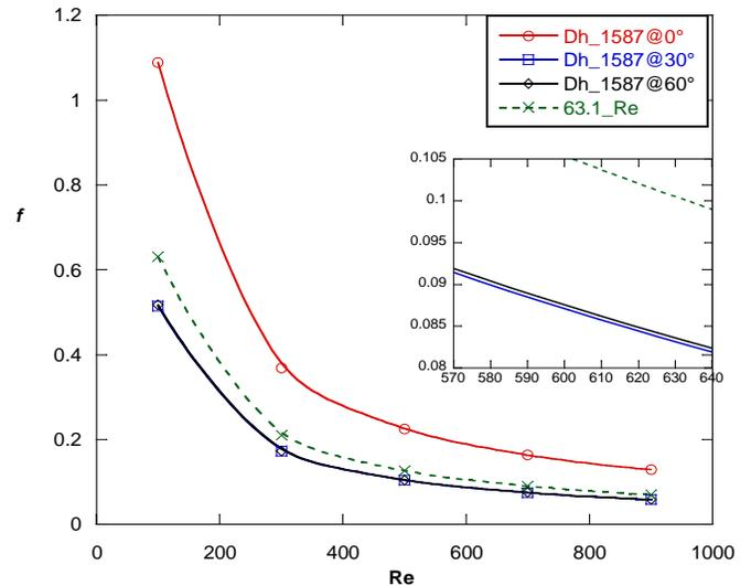
Fig. 6. Friction factor vs Reynolds number for Dh=1587 μm
