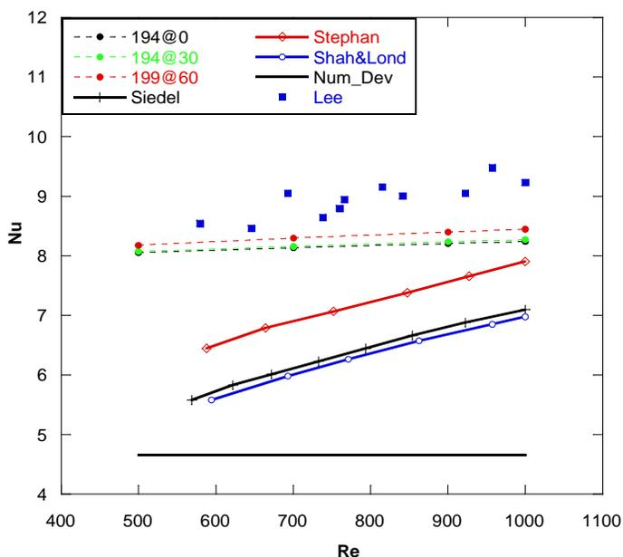
Fig. 7. Nusselt vs Reynolds number for Dh=199 μm
