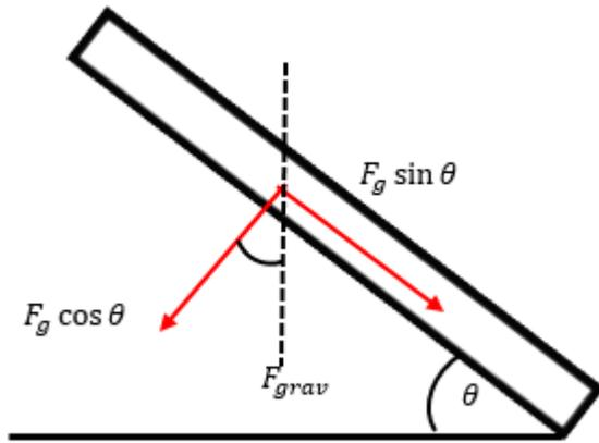
Fig. 2. Resolution of the gravity vector
