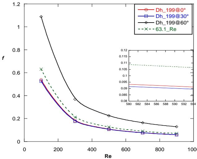
Fig. 4. Friction factor vs Reynolds number for Dh=199 μm
