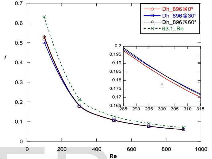
Fig. 5. Friction factor vs Reynolds number for Dh=896 μm
