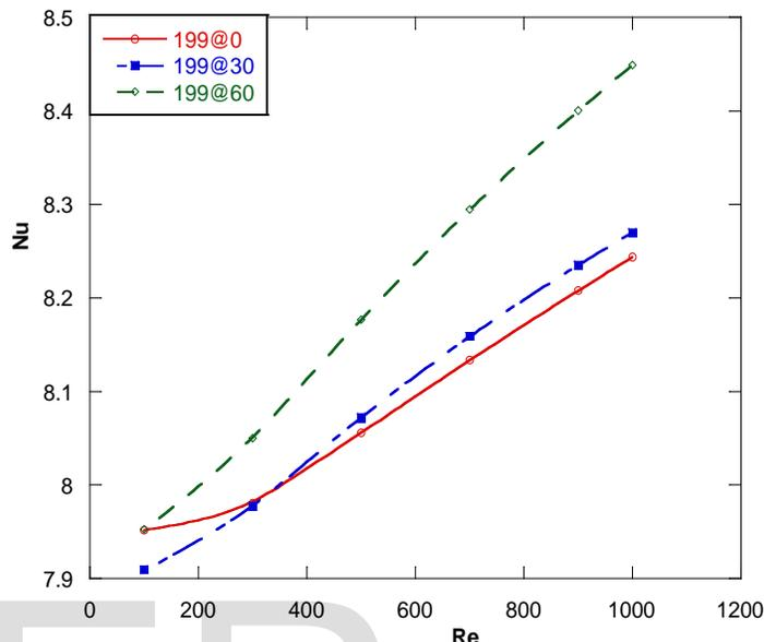
Fig. 8. Nusselt comparison for different angles with Dh=199 μm
