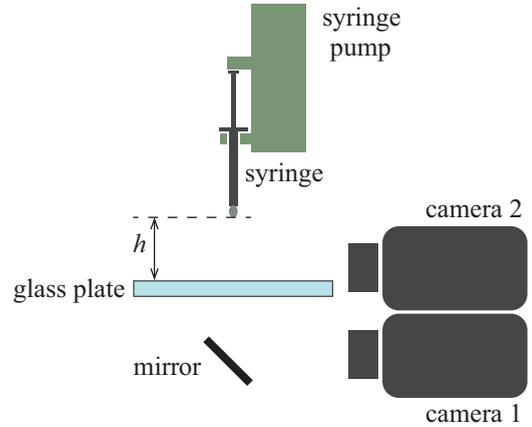
FIG. 3. Schematic view of the setup. Suspension droplets impact the glass plate at a speed  $U$ , set by the release height  $h$ . The ejection of particles and bouncing motion of the droplets upon impact is recorded using two high-speed cameras.
