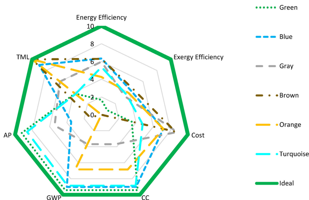
Fig. 12 – Overall performance comparison of selected hydrogen production color groups. (For interpretation of the references to color/colour in this figure legend, the reader is referred to the Web version of this article.)
