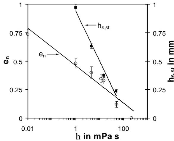
**Figure 9.** Effect of liquid viscosity on the restitution coefficient  $e_n$  of  $\gamma$ - $\text{Al}_2\text{O}_3$  granules (layer thickness of  $200 \mu\text{m}$ ) and on the sticking thickness  $h_{st}$ .
