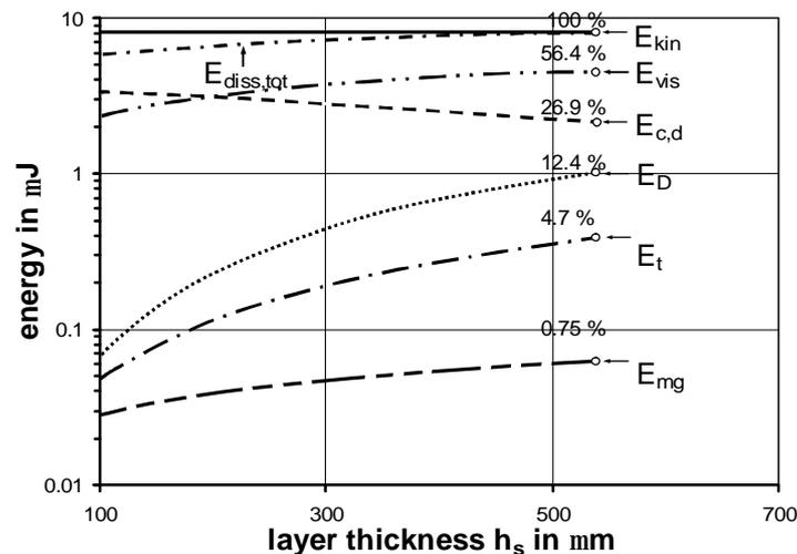
**Figure 12.** Kinetic impact energy ( $v = 2.36 \text{ m/s}$ ) and dissipated energy parts versus liquid layer thickness ( $h = 4.5 \text{ mPa}\cdot\text{s}$ ). The plotted values show the contribution of different energies at the sticking point.
