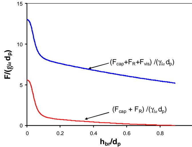
**Figure 13.** Comparison of the forces acting on the  $\gamma$ -Al<sub>2</sub>O<sub>3</sub> granule ( $d_p = 1.75$  mm) with the liquid bridge ( $h = 4.5$  mPa·s,  $g_a = 43.6$  mN/m) at static and dynamic conditions ( $v = 2.36$  m/s).
