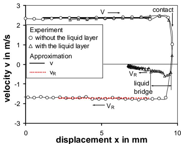
**Figure 7.** Approximation of the granule velocity before and after impact for typical velocity-displacement curves measured without a liquid layer and with a water layer of 700  $\mu\text{m}$ .
