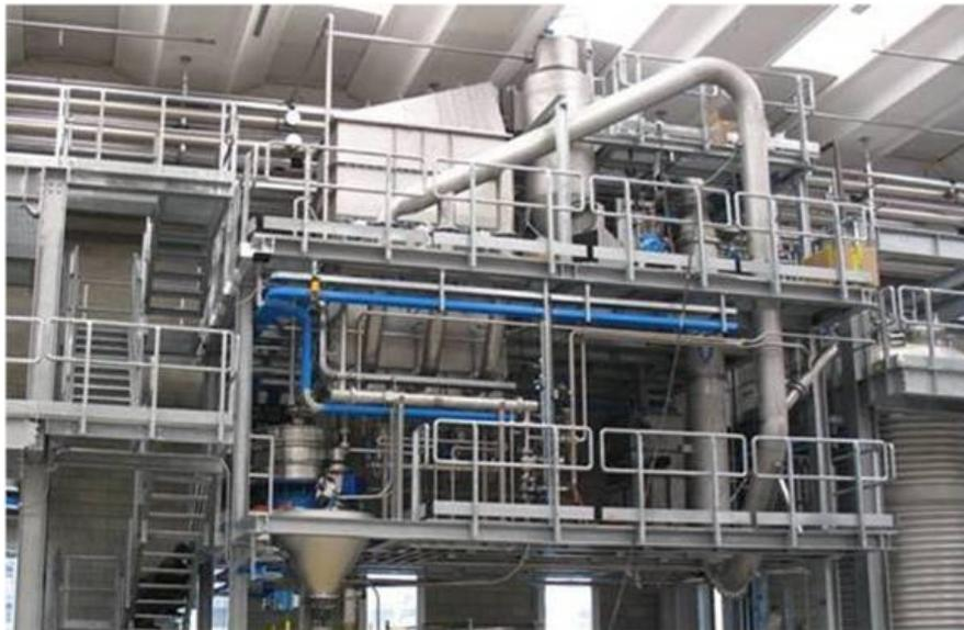
**Figure 11** Industrial scale granulation plant Glatt - ProCell 125 in closed loop operation (courtesy of Glatt/Germany).
