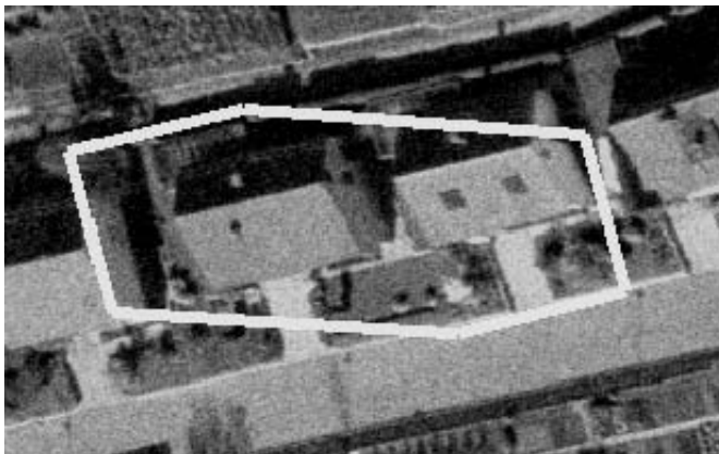
Figure 2.12: Localization of a building in case of large height variations of the terrain
