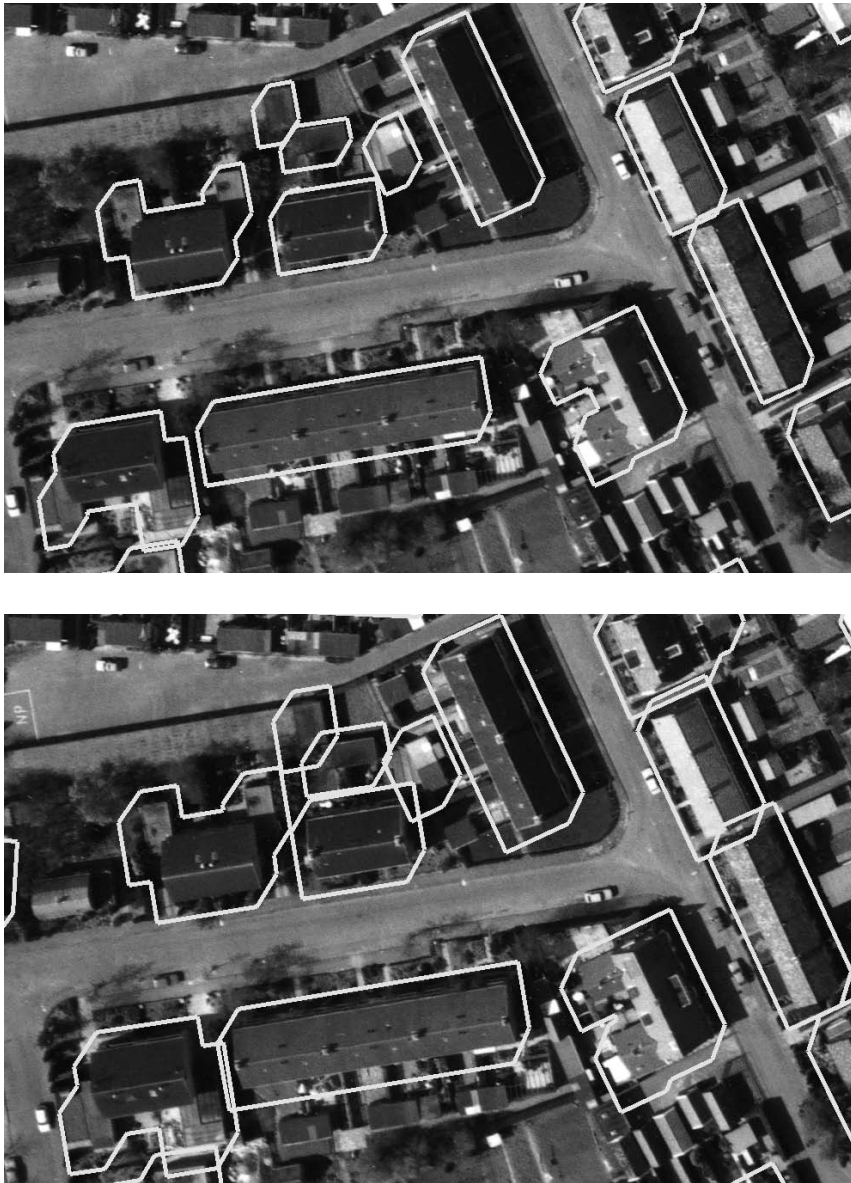
Figure 2.9: Localization of the buildings. Top contours after concatenation. Bottom contours after dilation
