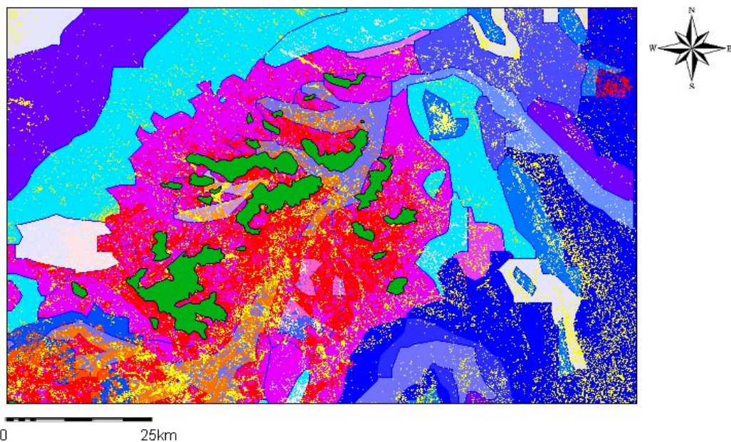
Figure 7.7. Overlain layers of gilgai soil and interpreted swelling based on spectral data (soil map 50%transparent)
