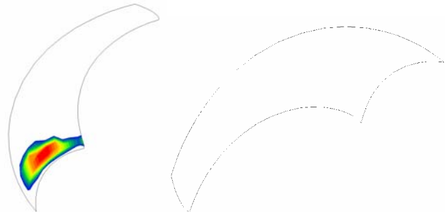
Figure 8 Sheet cavitation at the suction (left) and pressure (right) side of the impeller vane with asymmetric profiled vanes for \phi = 0.05 , \kappa = 0.031 .
