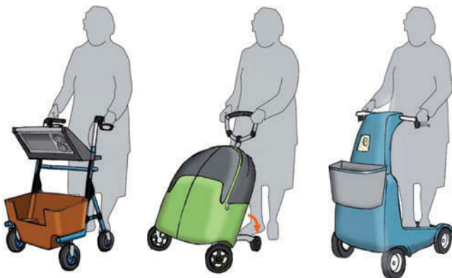
Figure 2. The three selected designs: left: the multifunctional wheeled walker, middle: the grow-along grocery bag, and right: the electric wheeled walker. For more details, see Appendix 2.
