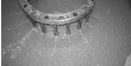
Figure 20: SCC after J-ring test with obvious flow marks behind the rods and around the spreading concrete.
