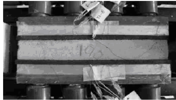
Figure 19: Sample holder of the thermal mass measuring device (sample between two thermo-regulated plates).
