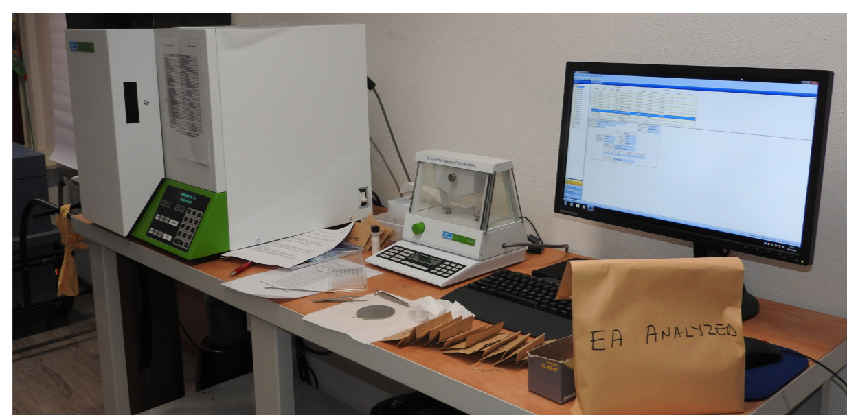
Figure 2: Dry combustion-reduction elemental analysis of leaf samples to determine foliar nitrogen and carbon.
