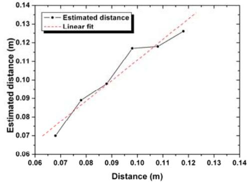
Fig. 6. Dipole source localization determined using the beamforming technique (dots) & linear fit between  $D$  and  $D_{\text{est}}$  (dashed line).
