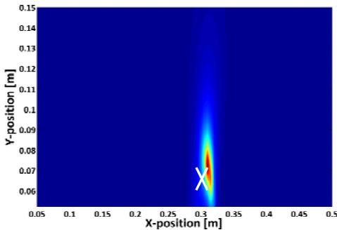
Fig. 5. Dipole source imaging using ALLS. Source positioned at  $x = 0.3$  m,  $D = 0.068$  m (white cross) and the estimated position is  $X_{\text{est}} = 0.31$  m,  $D_{\text{est}} = 0.072$  m. The red area indicates the area of increased likelihood of the source position.
