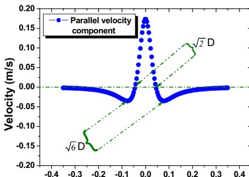
Fig. 2. Simulated velocity field  $V_{x//}$  (the parallel component) as function of sensor position along the LLS ( $x$ -axis). The LLS to dipole source distance ( $D$ ) is encoded within the characteristic points of dipole field.
