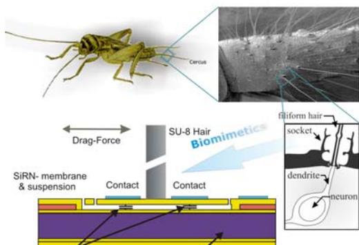
Fig. 1. Artificial hair geometry and its biological source of inspiration.
