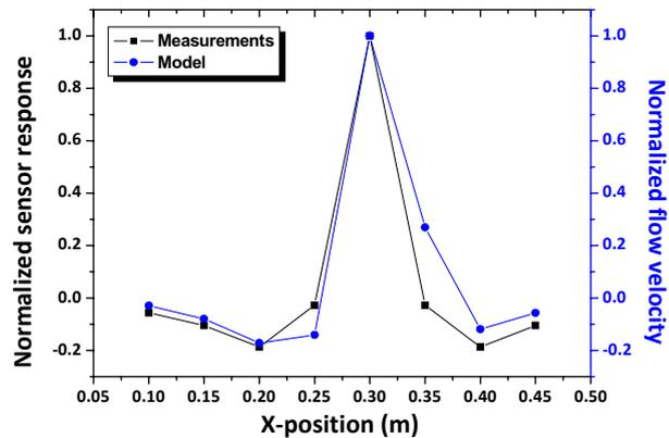
Fig. 4. Flow field measurements (as detected by 8 hair-sensors at  $x = 0.3$  m,  $D = 0.068$  m) versus theoretical model.
