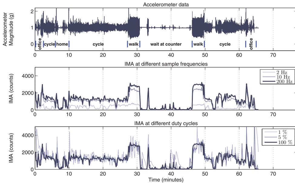
Fig. 2. IMA calculated from accelerometer data at various configurations
