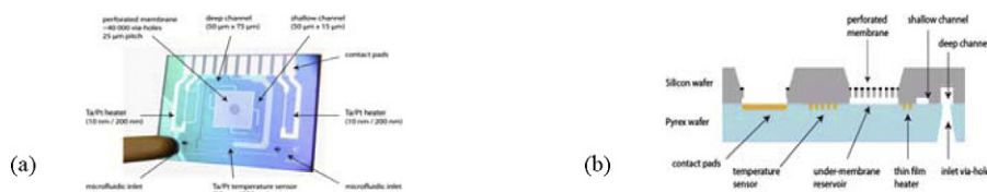
Fig. 1. (a) Evaporator image of the channel side; (b) schematic representation of its cross-section.
