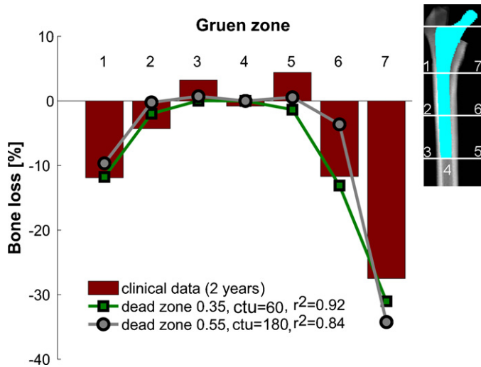
Fig. 3. Correlation results between the clinical (2 years in situ) data and data obtained from the remodeling simulations allowed us to define the best dead zone and real time.
