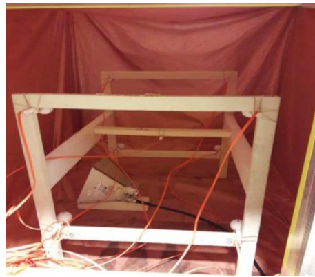
Fig. 2. Measurement setup with 9 electric field probes
