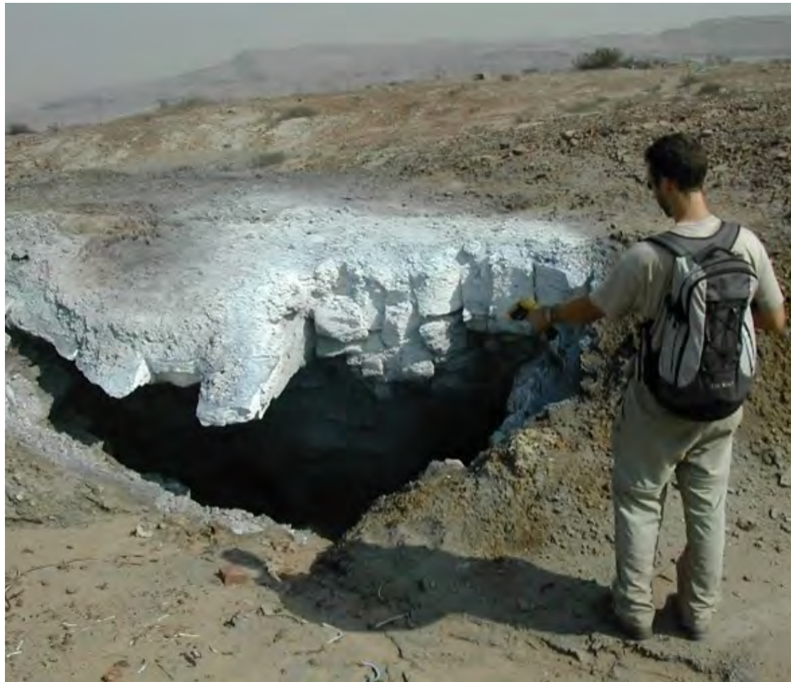
Figure 1: Ground truthing radiant temperatures of coal fire -related thermal anomalies detected from space over an area in Inner Mongolia, China in 2003.
