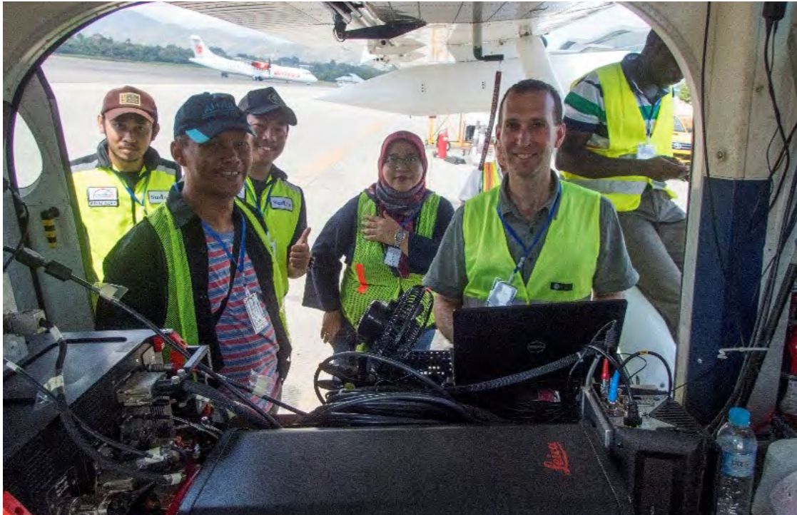
Figure 5: Part of the team from UT-ITC, U. Gadjah Mada, and airborne operator APG at the open hatch of the Pilatus Porter PC-6 at the Komodo International Airport, Indonesia (2018). The down-looking thermal broadband FLIR camera is visible between the Leica LiDAR head (big black box in center of image) and the water supply of the pilot (towards the right)
