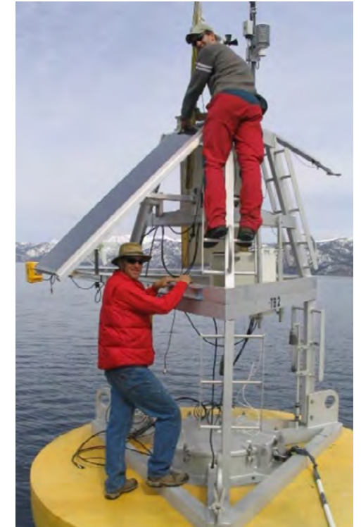
Figure 2: Maintenance visit to JPL's Lake Tahoe validation buoy for spaceborne TIR sensors with Simon Hook (not in the picture) and research staff from UC Davis in 2006.
