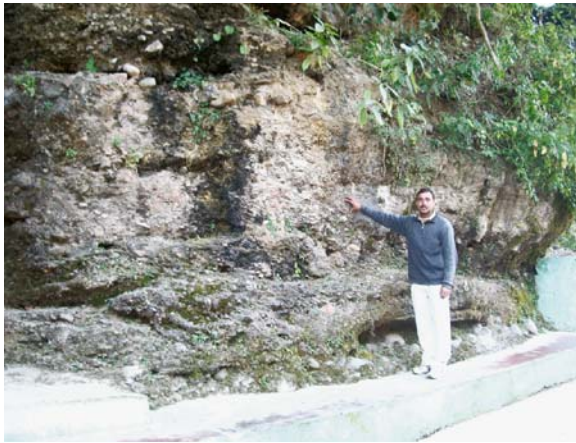
Fig. 6 Photograph near FRI site no. 26 showing the lithology below 10 m from the surface, which gives rise to V_s more than 350 m/s. At a depth of 30 m, the Doon gravels cemented with sandy calcareous materials show velocity more than 500 m/s
