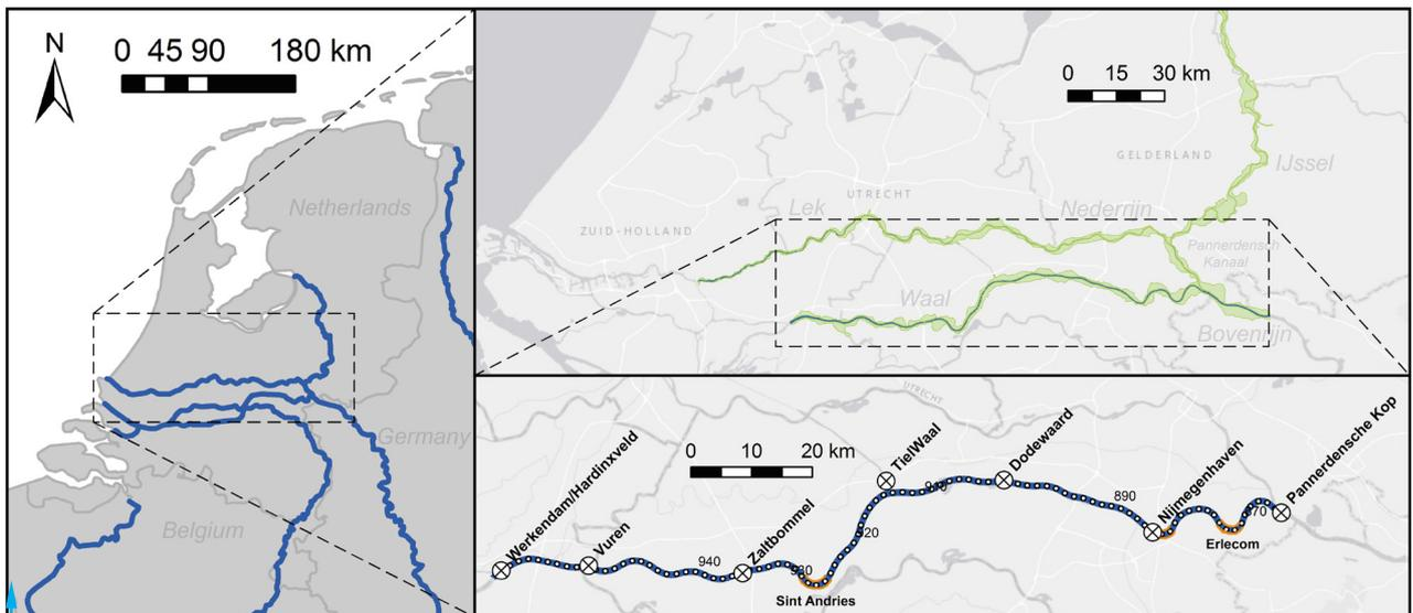
FIG. 2 Geographical overview of the River Waal in the Netherlands. Crossed circles indicate the location of water level observation stations. Orange highlighted areas indicate the location of submerged groynes or artificial armoured bed layers.
