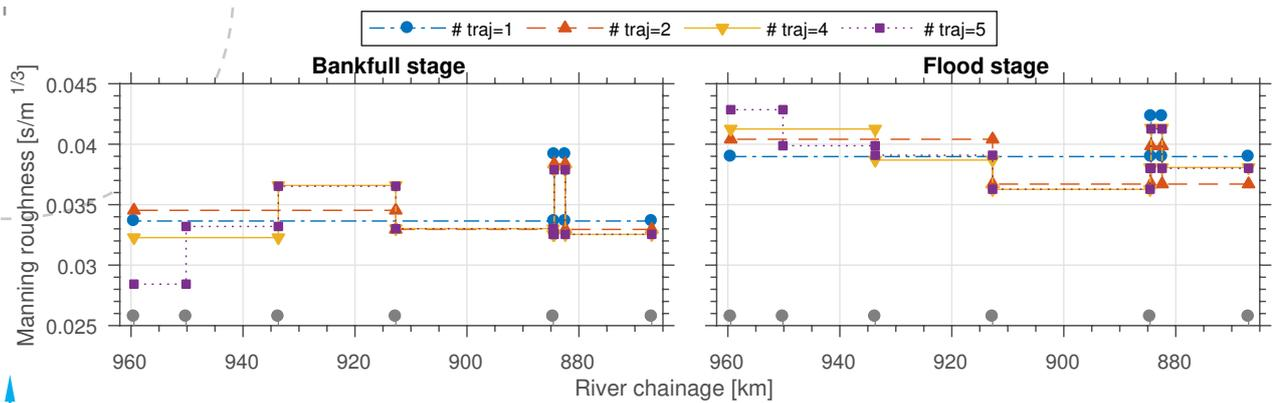
FIG. 4 Calibrated Manning roughness for varying number of roughness trajectories and for both bankfull and flood stage discharge peak. The grey dots right above the x-axis show observation station locations.
