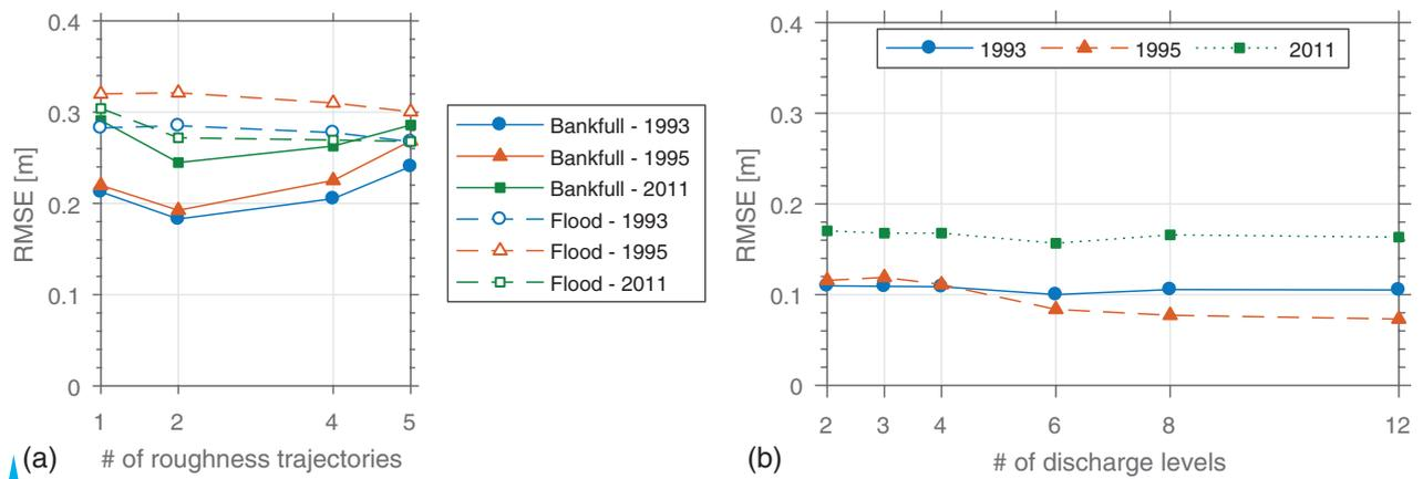
FIG. 6 a) Errors in water levels (RMSE), a) when calibrated on different number of roughness trajectories for bankfull discharge and flood discharge peak and b) when calibrated on different number of discharge levels
