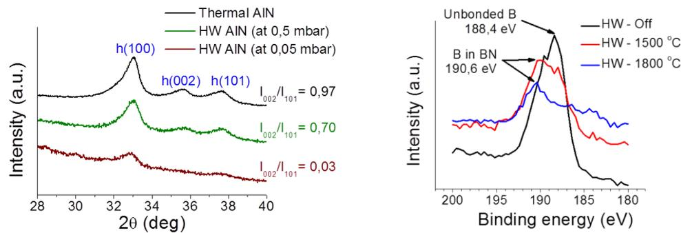
**Figure 3.** (Left) – GIXRD scans of thermal- and HW-deposited AlN: although both are hexagonal, the action of N-rad in HW-AlN lowered the  $I_{002}/I_{101}$  value. (Right) – Shift of the Boron 1s XPS peak with increasing HW temperature, indicating the transition from B-rich (N-deficient) films to BN films.
