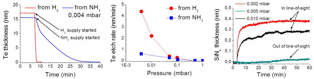
**Figure 1.** (Left, Center) – Etching of Te films by at-H from the dissociation of H<sub>2</sub> and NH<sub>3</sub> on HW at 1800 °C. (Right) – Nitridation of (H-terminated) Si wafers under different pressures by N-containing radicals, as generated from HW-dissociated NH<sub>3</sub>. Further, nitridation in- and out-of-line-of-sight-of-HW were compared.
