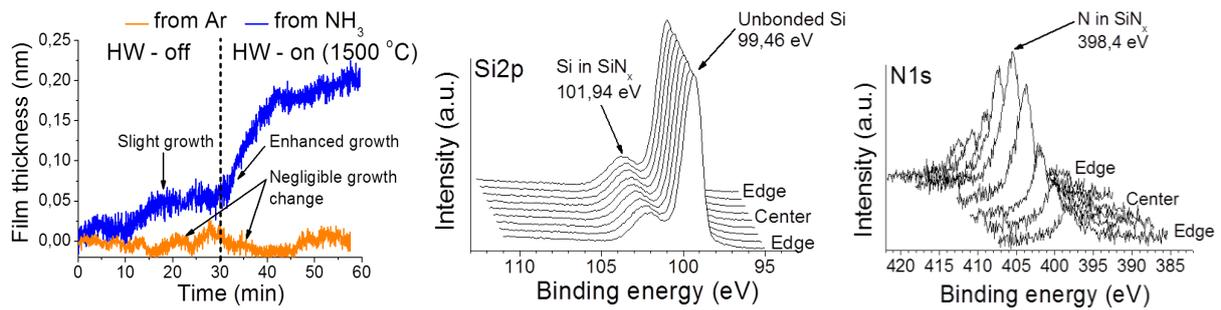
**Figure 2.** (Left) – Replacing NH<sub>3</sub> by Ar showed no film growth (orange) hence indicating film formation by Si-nitridation over Si-oxidation by HW-dissociated NH<sub>3</sub> (blue). (Center, Right) – XPS survey scans confirmed the formation of SiN<sub>x</sub> with the highest N-concentration at the center of the wafer (i.e. in the line-of-sight).
