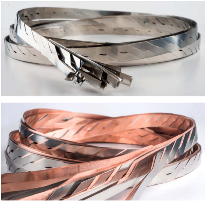
Fig. 6. Samples of Roebel dummy cables produced within the scope of the EuCARD2 activities: (top) SS tape and (bottom) assembly of SS and Cu tapes.
