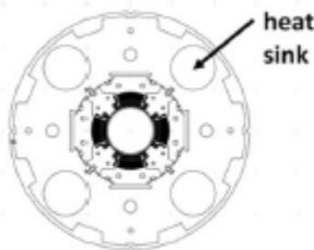
Figure 1 quadrupole magnet cross-section
