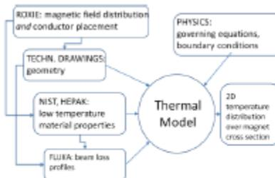
Figure 2 Schematic overview of thermal model
