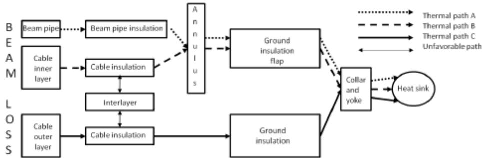
Figure 4 Thermal paths from heat source to heat sink
