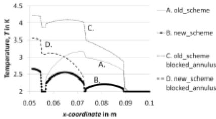
**Figure 7** Temperature profile through the middle of the midplane conductors radially outward
