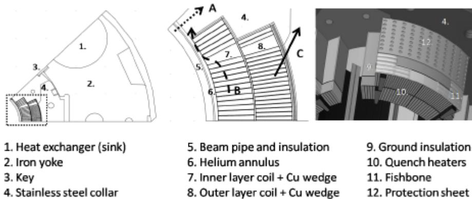
Figure 3 (left) quadrupole octant, (middle) zoom of the coil, (right) 3D representation
